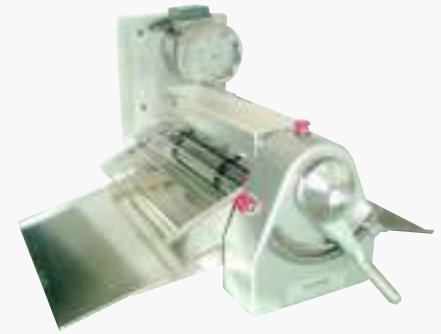
Pastry Brakes are good for bakeries with confined spaces, these are essentially the same machine as the pastry sheeter, but without the belts.
