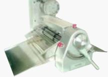
Pastry Brakes are good for bakeries with confined spaces, these are essentially the same machine as the pastry sheeter, but without the belts.
