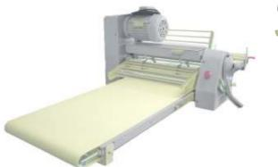
The dough thickness has a locking scale with a final thickness stopper. One of the most unique features of these sheeters is that they offer a single line tracking system in order to eliminate belt wander.
